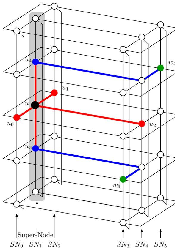
Figure 4: Distributing image on  $2 \times 3 \times 5$  Torus
