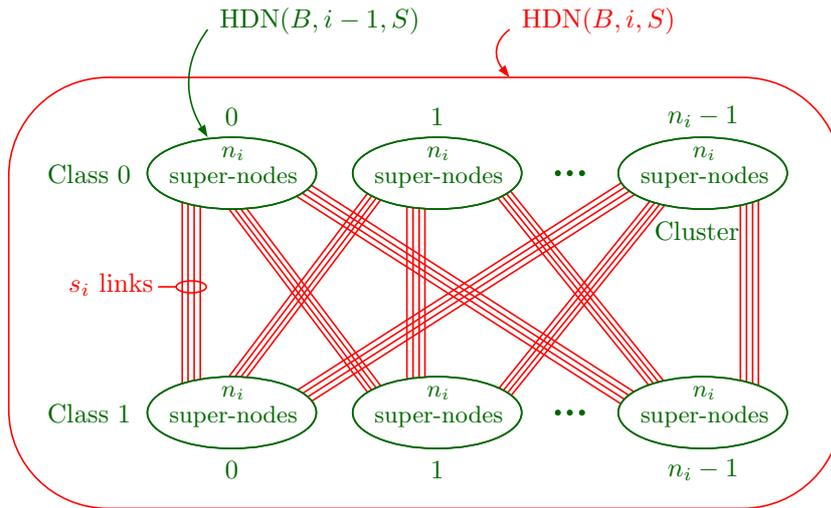
Figure 1: Build an  $HDN(B, i, S)$  from  $HDN(B, i - 1, S)$  [6]
