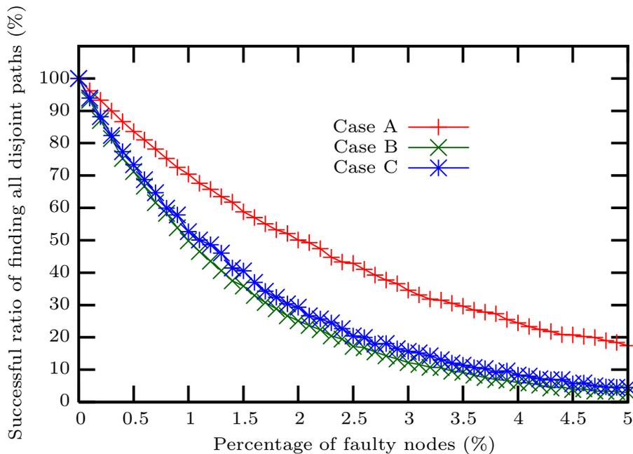
Figure 12: Successful ratio of finding all disjoint-paths
