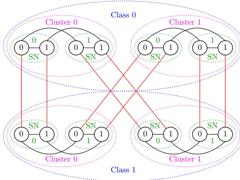
Figure 2: An  $HDN(B, 1, S)$  with  $s_1 = 2$  [6]
