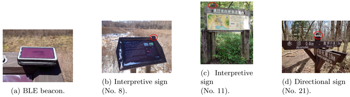
Figure 2: BLE beacons and their installation at guide points (beacon locations indicated by red circles).
